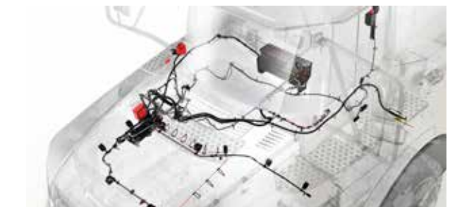
Volvo fire suppression system
