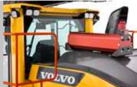
Fire suppression system
