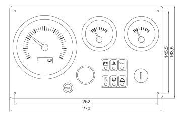
$Key, start \ button, acoustic \ alarm, analogue \ instruments \ (revolution \ counter, water \ temperature, oil \ pressure), LCD \ display \ alternating \ voltmeter \ and \ hour \ counter, warning \ lamps \ (oil \ pressure, water \ temperature, \ alternator \ charger, \ glow \ plugs, \ water \ presence \ in \ the \ fuel, \ generic \ alarm), \ fuse.$
