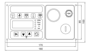
Key, start button, acoustic alarm, digital indicator (rpm counter, hour counter, water temperature, voltmeter), warning lamps (oil pressure, water temperature, alternator, glow plugs, low battery voltage), fuse.
