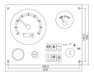
Key, start button, acoustic alarm, analogue instruments (revolution counter, water temperature), LCD display alternating voltmeter and hour counter, warning lamps (oil pressure, water temperature, alternator charger, glow plugs, water presence in the fuel, generic alarm), fuse.
