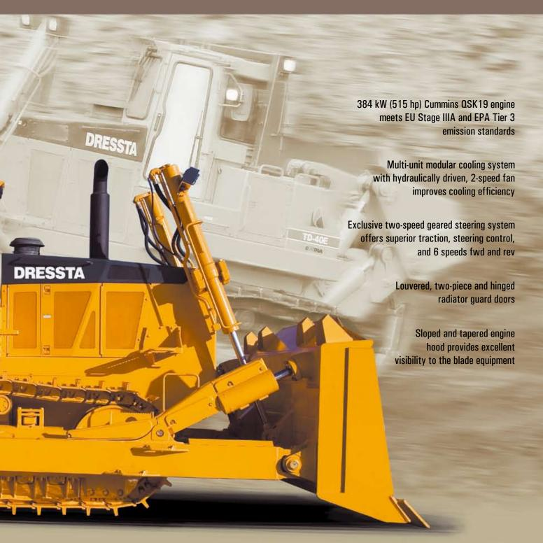
ign provides maximum durability ator a smoother, stable ride Large capacity blades with full width wear liner and double tilt/pitch system, for all types of dozing operations
