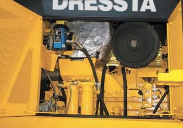
The Tier 3 approved Cummins QSK19 engine with state-of-the-art electronic controls and modular common-rail fuel system ensures clean, efficient performance, minimum maintenance and superior uptime.
