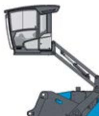
Cab system hydraulically adjustable
