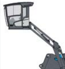
Cab system vertically adjustable and horizontally adjustable
