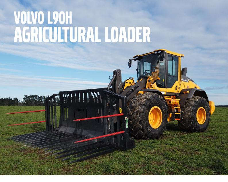
The powerful Volvo L90H wheel loader is built for a variety of applications, including quarrying, timber handling, and agriculture. Volvo's Torque Parallel-linkage, hydraulic attachment bracket, and range of attachments really do make the L90H the ultimate all-rounder. The optional 8m3 folding silage fork and Michelin Mega Xbib Ag tyres, ensures the Volvo L90H Agricultural Loader is a highly productive, extremely versatile tool for all applications on or around the farm.
