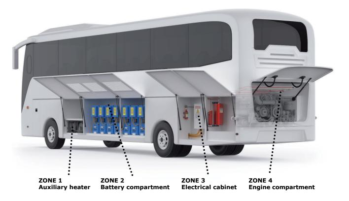
The different protection zones are then protected in various ways by robust detection and suppression systems – both liquid based and gas-based solutions.
